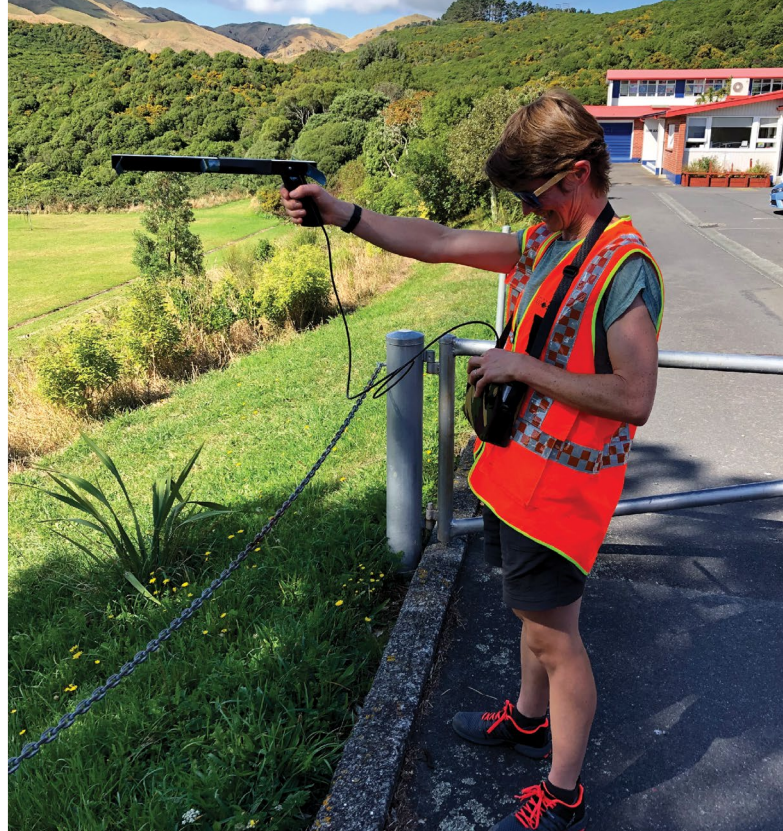
Using a receiver to pick up a specific radio frequency from a Wander Search pendant.
